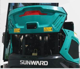
YANMAR Engine with slide up access panel for maintenance
